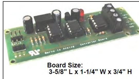
Figure 25: Servo to Analog Conversion Board by Blue Point Engineering
