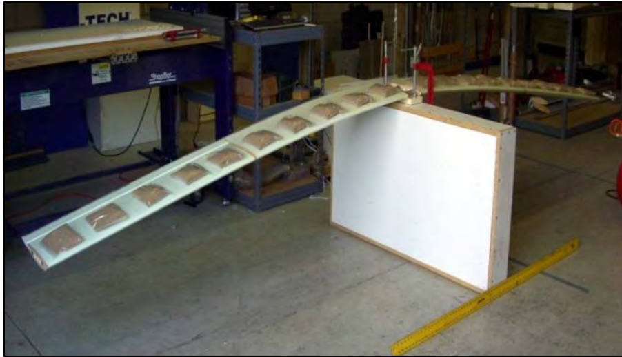
Figure 16: CLMax Wing Loading Tests (15-ft Wingspan)
